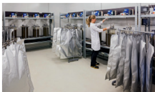
Continuous biogas fermenters – from basic research in batch fermenters and trials in continuous fermenters through to field studies in parallel working commercial fermenters, the ISF Schaumann Research has created outstanding facilities for resolving complex issues relating to biogas production.
