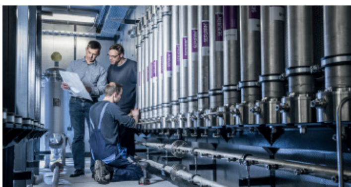
Production in Zeven – Assembly of a plant using membrane-based gas permeation
