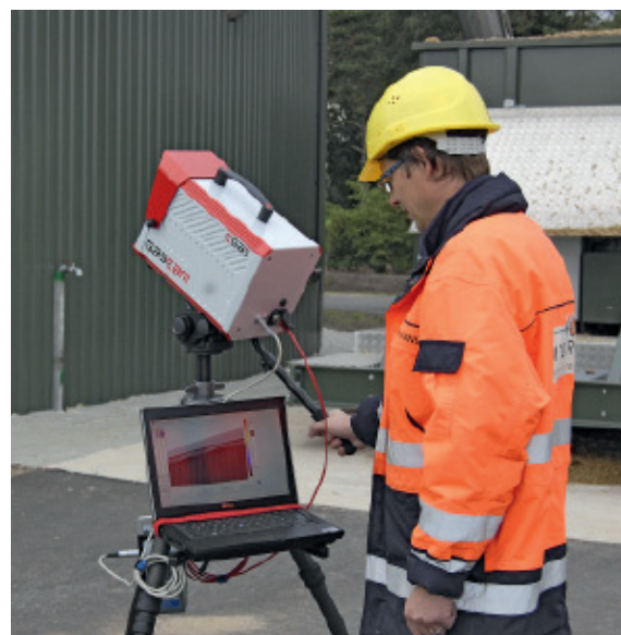
Gas leak detection during the maintenance
